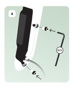
↑ Tighten the two screws into the motor cable cover (2Nm). Make sure both of them are secure.
