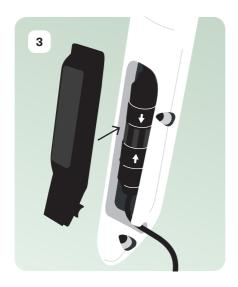
↑ Push the cable and connector into the fork leg and put the plastic cover over the motor cable notch on the front fork.
