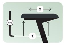
↑ Loosen both screws underneath the saddle, adjust the seat to your preferred position, and tighten the screws (10Nm).
