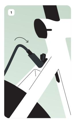
v Open the rubber cover located between the rear stays and gently insert the charging plug in the charging port.
