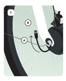
↑ The motor cable must go around the back of the fork, between the fender stay (A) and the spokes (B).
