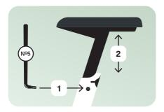
↑ Remove the rubber cap and loosen the screw. Slide the seat to your preferred height, tighten the screw (10Nm), and put the rubber cap back on.
