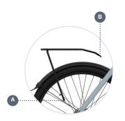
Finally, tighten the carrier stay bolts, using Allen key #3. Now the rear carrier is ready to be used!
