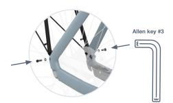
Tighten the 20mm bolt to the tube located underneath the rear light (B), using Allen key #3. Make sure to place the washer between the frame and the carrier.
