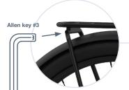
Tighten the two 16mm bolts, including washers, in the lower ends (A) using Allen key #3. Make sure the carrier stays are on the inside of the rear drop-outs.
