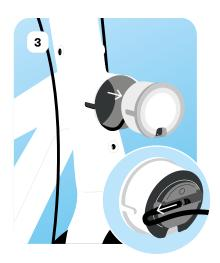
↑ Wiggle the front light out and unplug the connector from behind the light.
