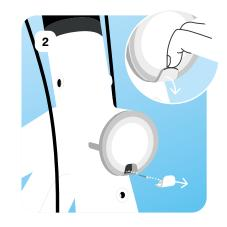
↑ Push down and remove the small plastic lens under the front light. Remove the screw using the Torx key Nº10.
