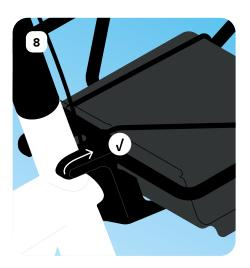
↑ Ensure all three screws are properly aligned, then fully tighten them with the Allen key Nº5. Put the two rubber covers back to cover the top screws.
