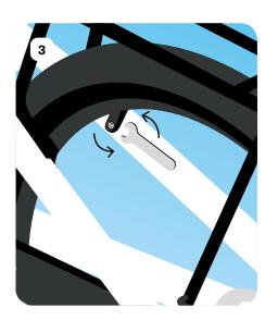
↑ Fully tighten the two hex head screws using the wrench.
