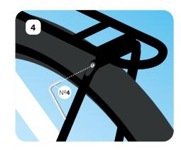
↑ Tighten the rack stay screws using Allen kev Nº4.
