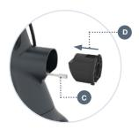
**1.5** Screw the M5\*25 bolt with Allen key #3 to the frame.
