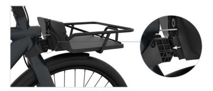
3.2 Tighten the M8\*20 bolt (including washer) to mount the main plate to the adapter, using Allen key #5.
