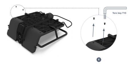
**A.2** Remove the back covers from the main plate. The loop of the elastic cords should remain around the outside screw studs (F).
