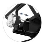
4.2 Gently pull the cable towards the front of the product, and stow away recess cable inside the light cover. Now slide in the front light (A) and fixate it with the set-screw, using anti-theft Torx #T10. (B).
