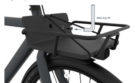
3.3 Mount the two M6\*15 bolts with Allen key #5 (including washers) to fixate the main plate to the bracket.
