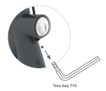
**1.3** Slide the front light out of the frame (A) and unplug the connectors (B).
